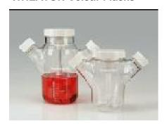
WHEATON Celstir Spinner Flasks features an adjustable paddle blade impeller for better mixing. The addition of the bottom dimple to flasks 125 mL and larger improves circulation and reduces the accumulation of cells in the center of the flask. Celstirs provide maximum surface interface between culture and flask atmosphere. Use the Celstirs for microcarrier and suspension cultures such as insect cells, hybridomas and adapted cell lines.
